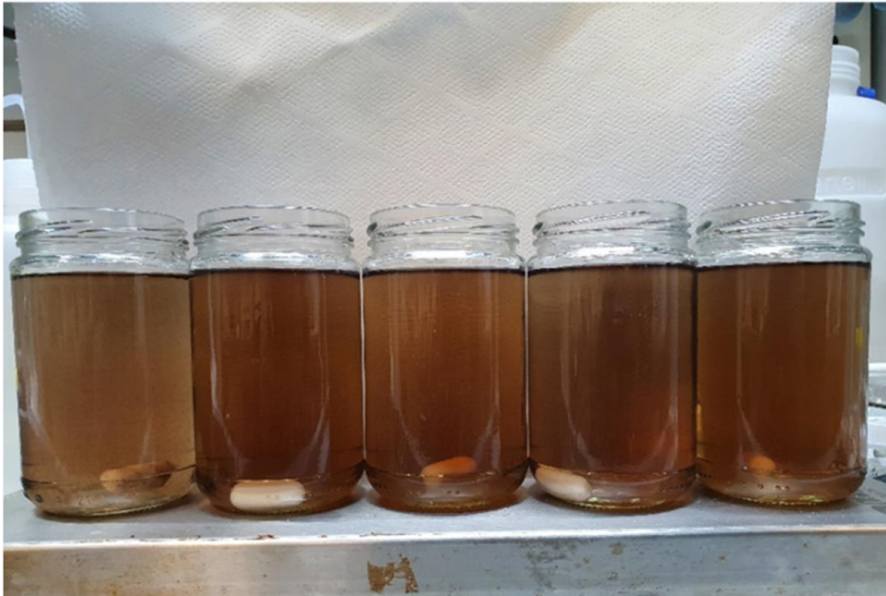
PbS test (t=0 and t=2h respectively). From left to right: Blank, Competitor, SPE2122 A, SPE2122 B, SPE2122 C
